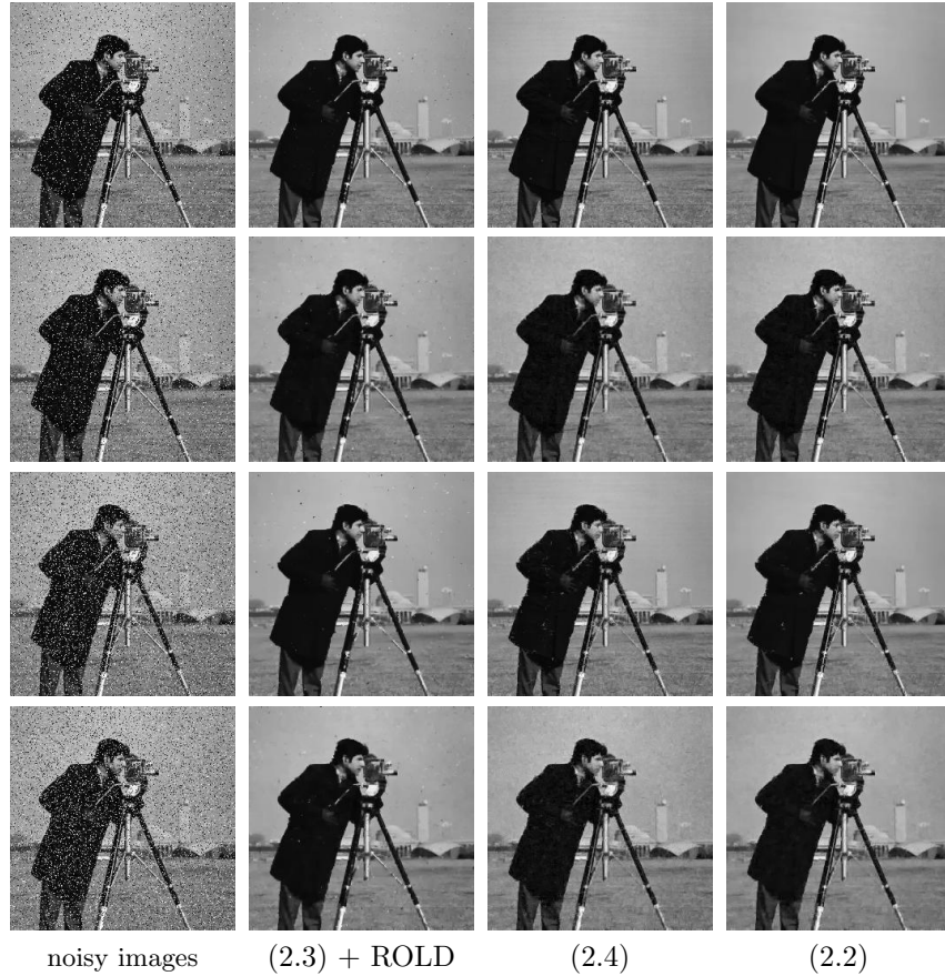
Figure 1: Denoising results of cameraman image contaminated by both random-valued impulse noise and Gaussian noise. Images in each column represent (from left to right) corrupted images, results from (2.3) combined with ROLD pre-detection, results from (2.4) and results from (2.2) respectively. The noise levels of corrupted images (from top to bottom) are as follows. (1) 10% random-valued impulse noise without Gaussian noise; (2) 10% random-valued impulse noise with Gaussian noise of \sigma=10 ; (3) 20% random-valued impulse noise without Gaussian noise (4) 20% random-valued impulse noise with Gaussian noise of \sigma=10 . The PSNR values of the results are given in Table 1.
