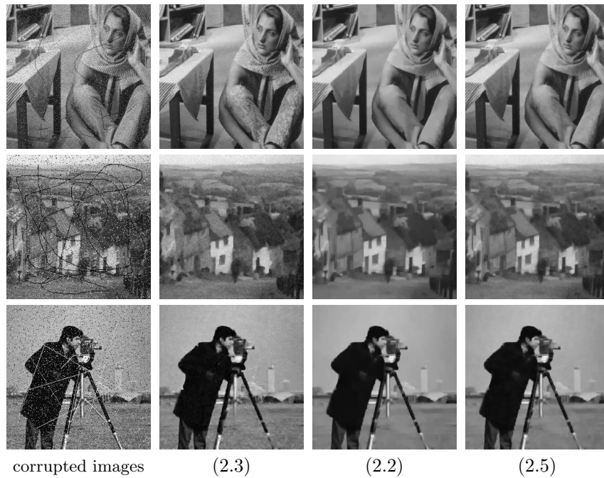
Figure 4: The blind inpainting results for images damaged by both impulse noise, scratch and Gaussian noise with \text{std}=10 . Three sample images are shown (from top to bottom): "Barbara", "goldhill" and "cameraman". Images in each column represent (from left to right) corrupted image, restored image by (2.3) with ROLD pre-detector, restored image by (2.2) and restored image (2.5). The PSNR values of the results are given in Table 4.
