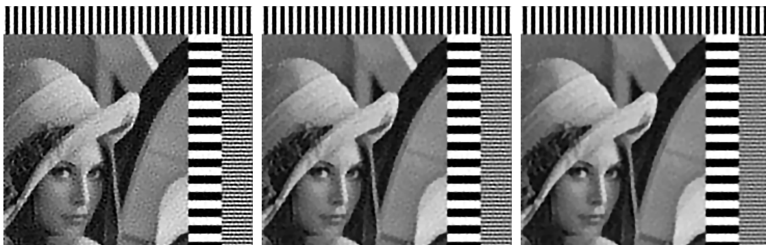
Figure 5: Recovered “lena” by the split Bregman algorithm with \lambda = 0.1, 0.2 and 0.3 respectively, and the corresponding PSNR values are 22.26, 20.42 and 18.25.
