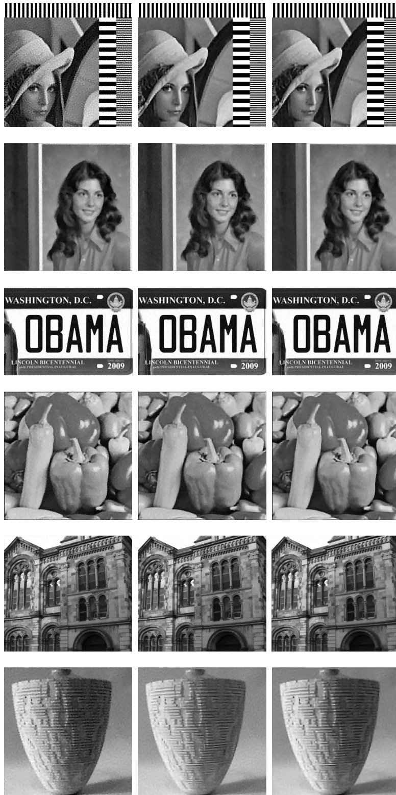
Figure 3: Image deblurring results of the split Bregman algorithm (left column), the PD method (middle column) and the MDAL method (right column). Noise level: \sigma = 4 .
